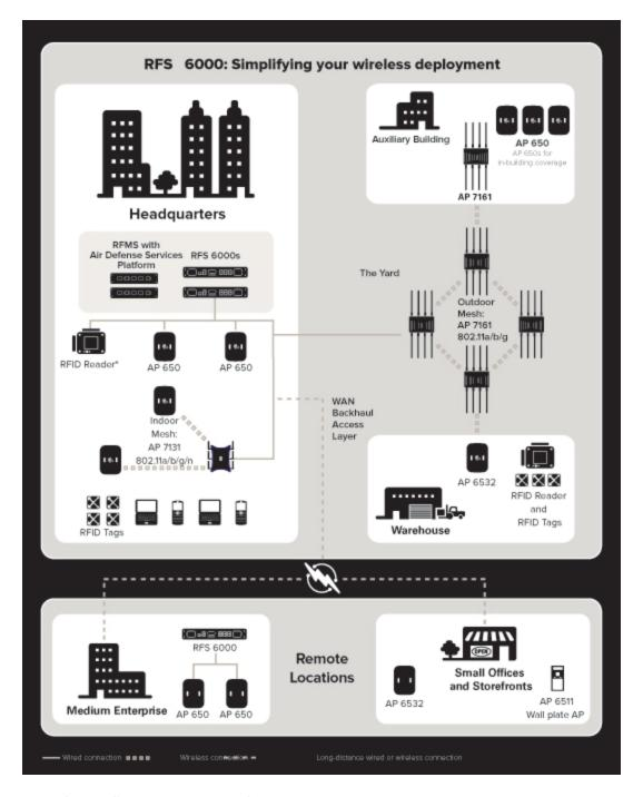
The RFS 6000 offers the comprehensive functionality necessary to extend wireless voice, video and data access inside medium to large enterprises — as well as to remote locations such as branch offices.
